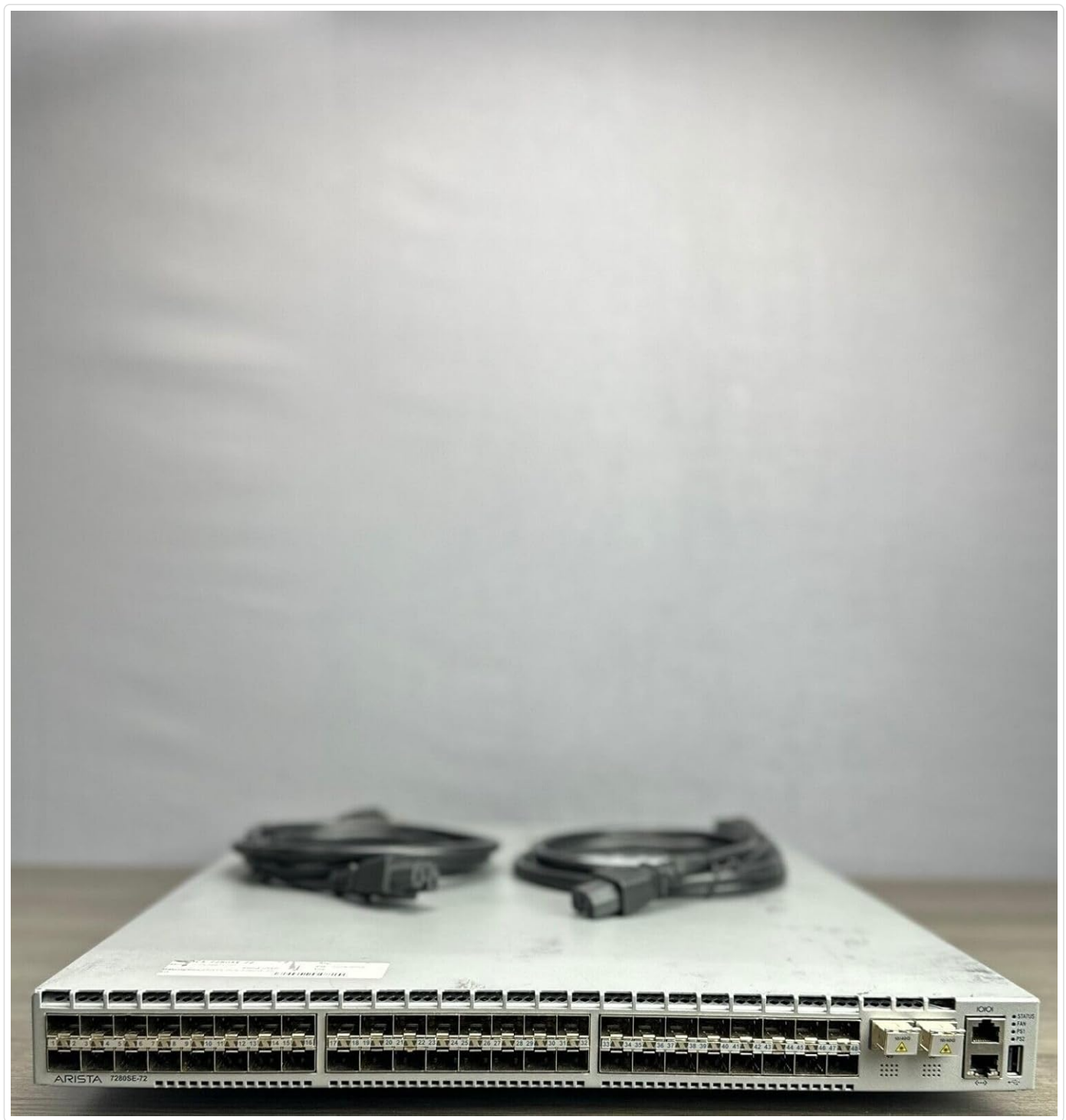
Figure 1: Front view of the Arista DCS-7280SE-72 Ethernet Switch. This image displays the front panel of the switch, highlighting the 48 SFP ports for various fiber optic connections and the two high-speed 100 Gigabit Ethernet uplink ports, along with status indicators.
