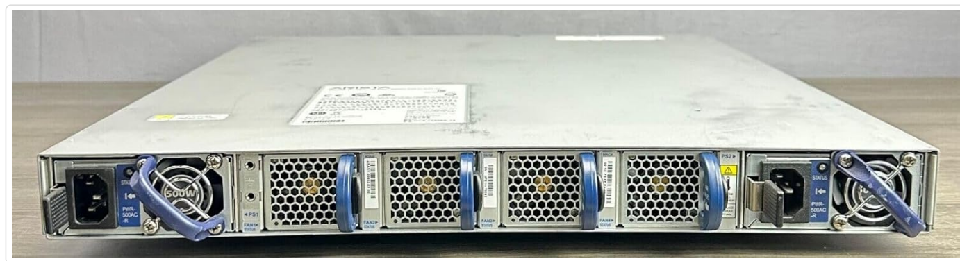
Figure 2: Rear view of the Arista DCS-7280SE-72 Ethernet Switch. This image illustrates the rear panel, featuring multiple modular power supply bays and fan units, designed for redundancy and ease of maintenance.
