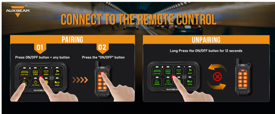
Figure 2: Remote Control Pairing Process. This diagram illustrates the two-step process for pairing the wireless remote with the switch panel.
