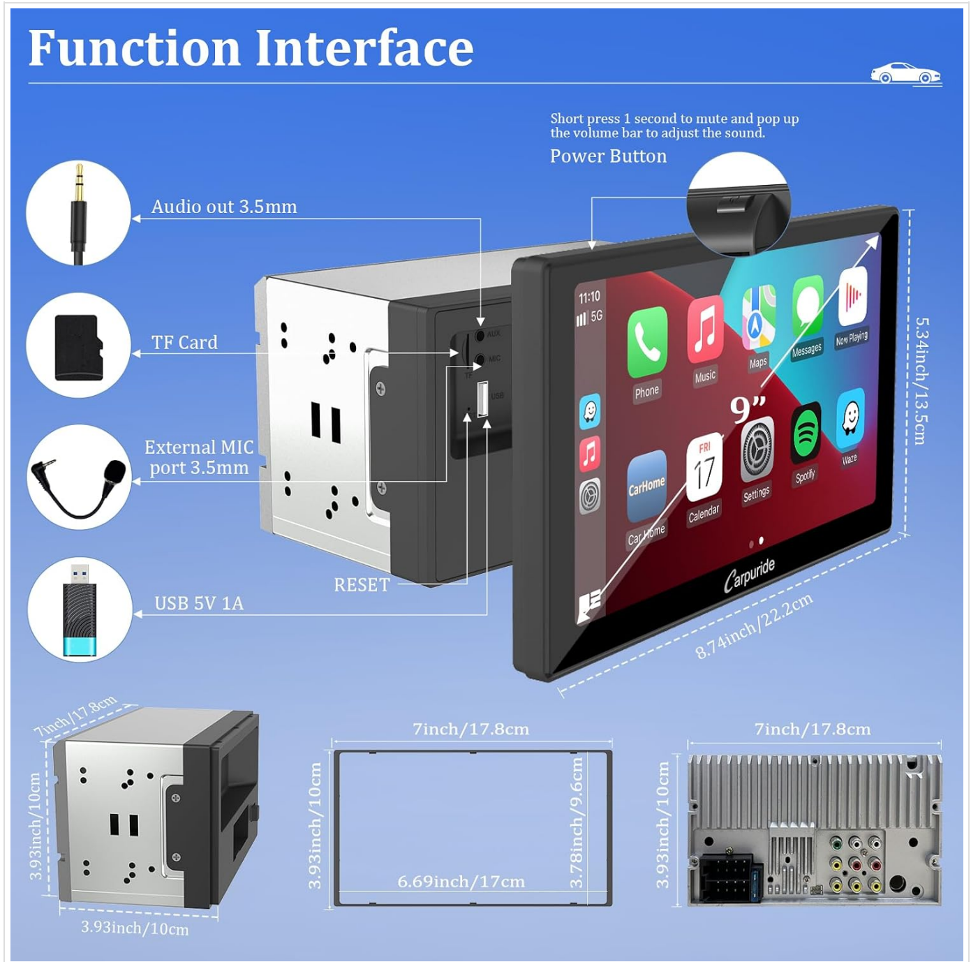
Image: Front and rear views of the Carpuride car stereo, highlighting the 9-inch detachable screen, audio out 3.5mm, TF card slot, external MIC port 3.5mm, USB 5V 1A, RESET button, and various rear wiring connections with dimensions.
