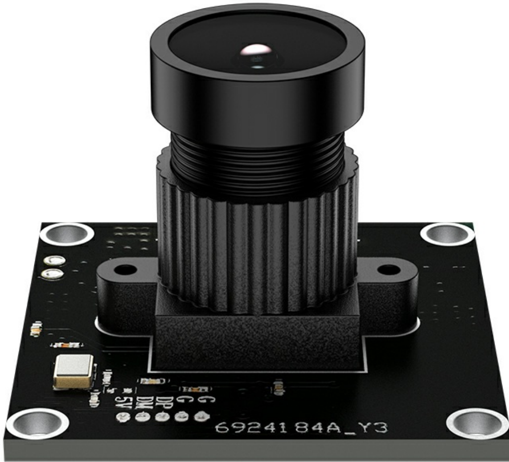
Figure 2.1: Front-angle view of the InnoMaker camera module, showcasing its compact design and integrated lens.
