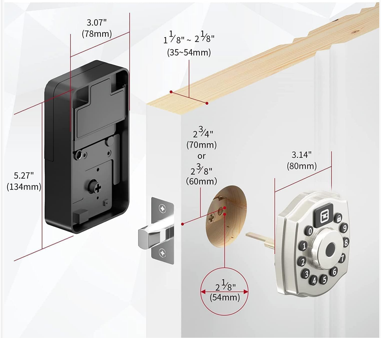
Figure 3.1: Detailed dimensions for door preparation, including measurements for the latch, exterior panel, and interior panel.
