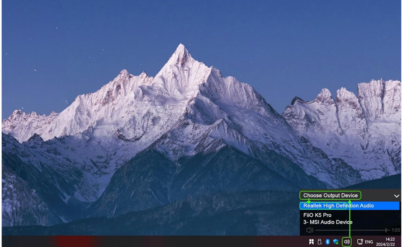
Image: A screenshot demonstrating how to select the SOULION R30 speaker as the audio output device in Windows, showing the speaker icon and the "Choose Output Device" menu.
