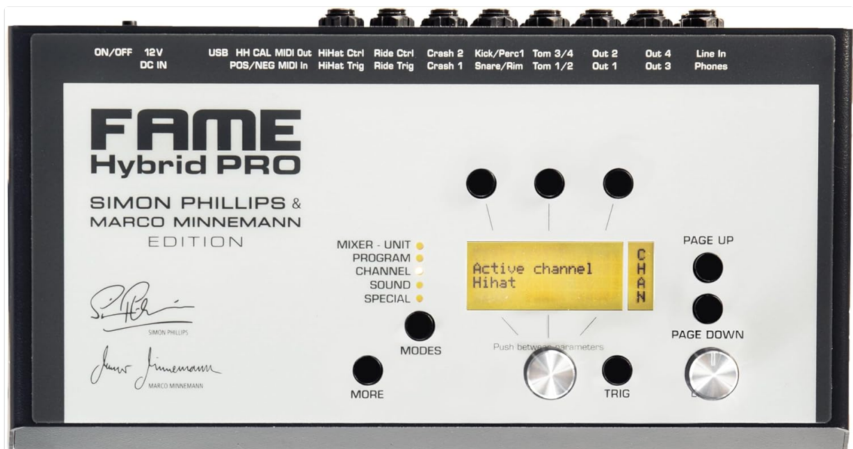
Image 5.2: Display showing 'Active channel Hihat' in CHANNEL mode, indicating trigger settings for the hi-hat.
