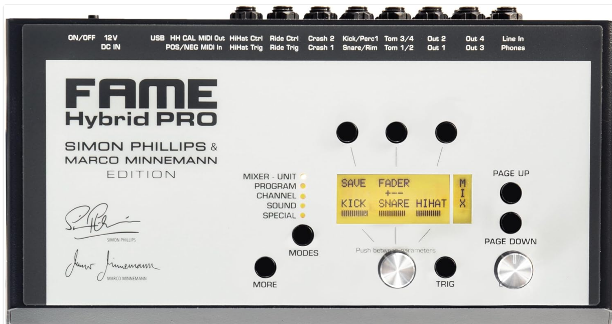
Image 5.5: Display showing 'SAVE FADER MIX' in MIXER - UNIT mode, indicating options for saving kit mixes and adjusting fader levels.
