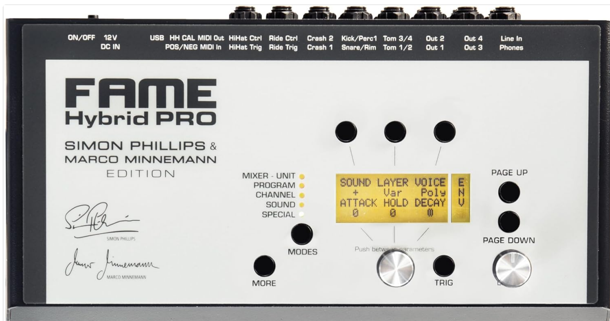
Image 5.3: Display showing 'SOUND LAYER VOICE' parameters in SOUND mode, allowing detailed voice editing.
