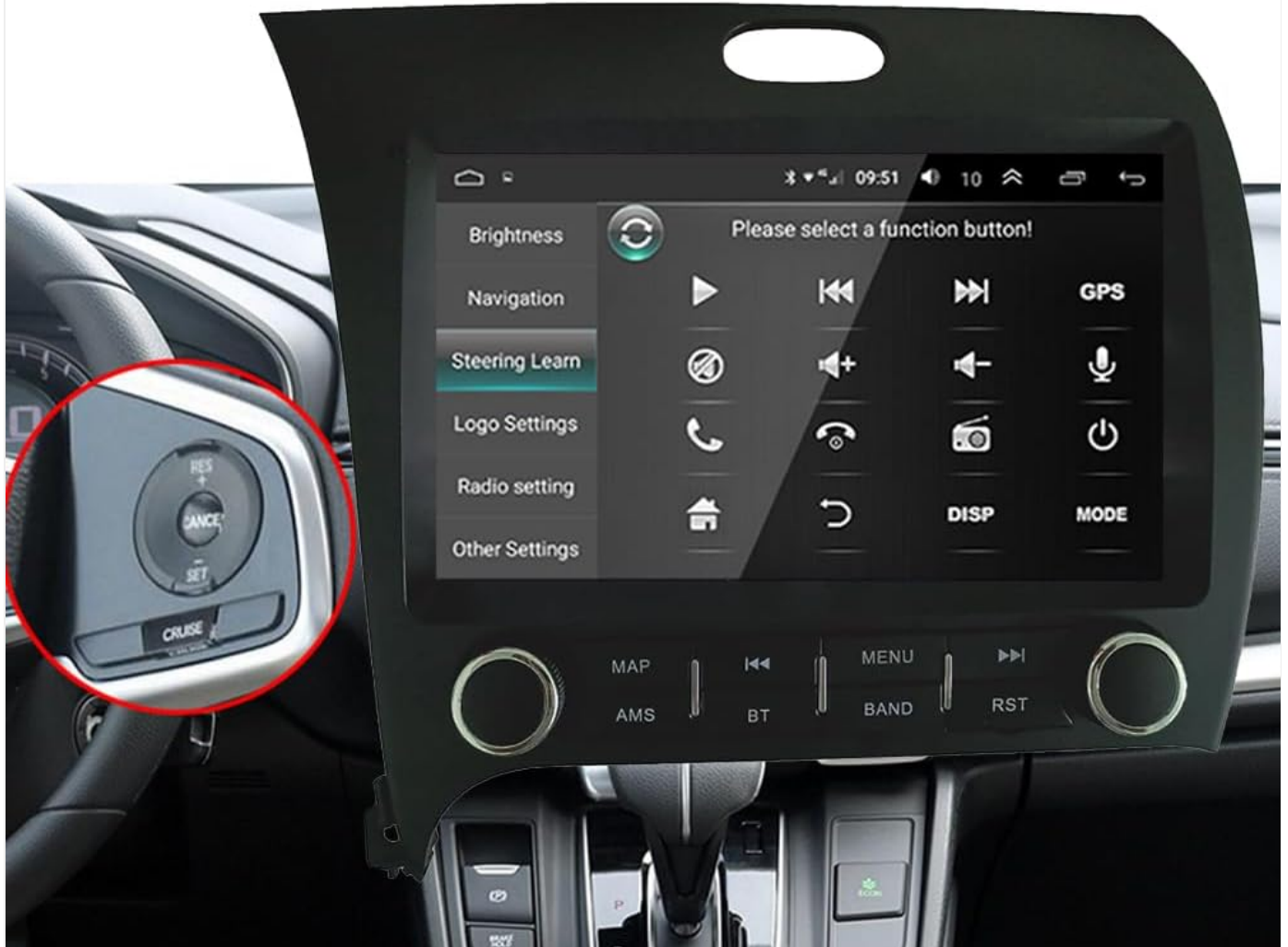
Image: The head unit displaying the "Steering Learn" menu, with an inset showing a car's steering wheel controls.
