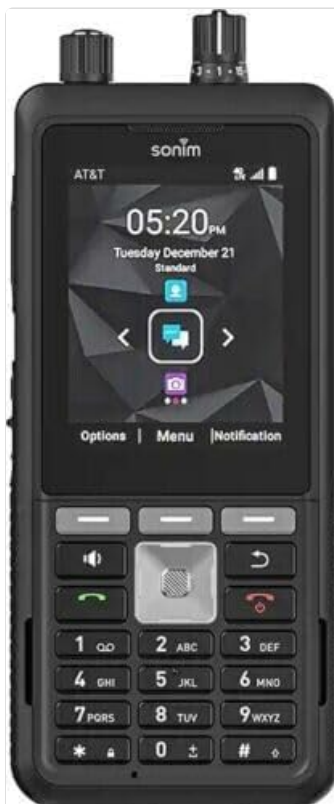
Image: A close-up front view of the Sonim XP5 Plus, highlighting the screen interface, the physical keypad, and the two rotary knobs located at the top of the device for channel and volume control.
