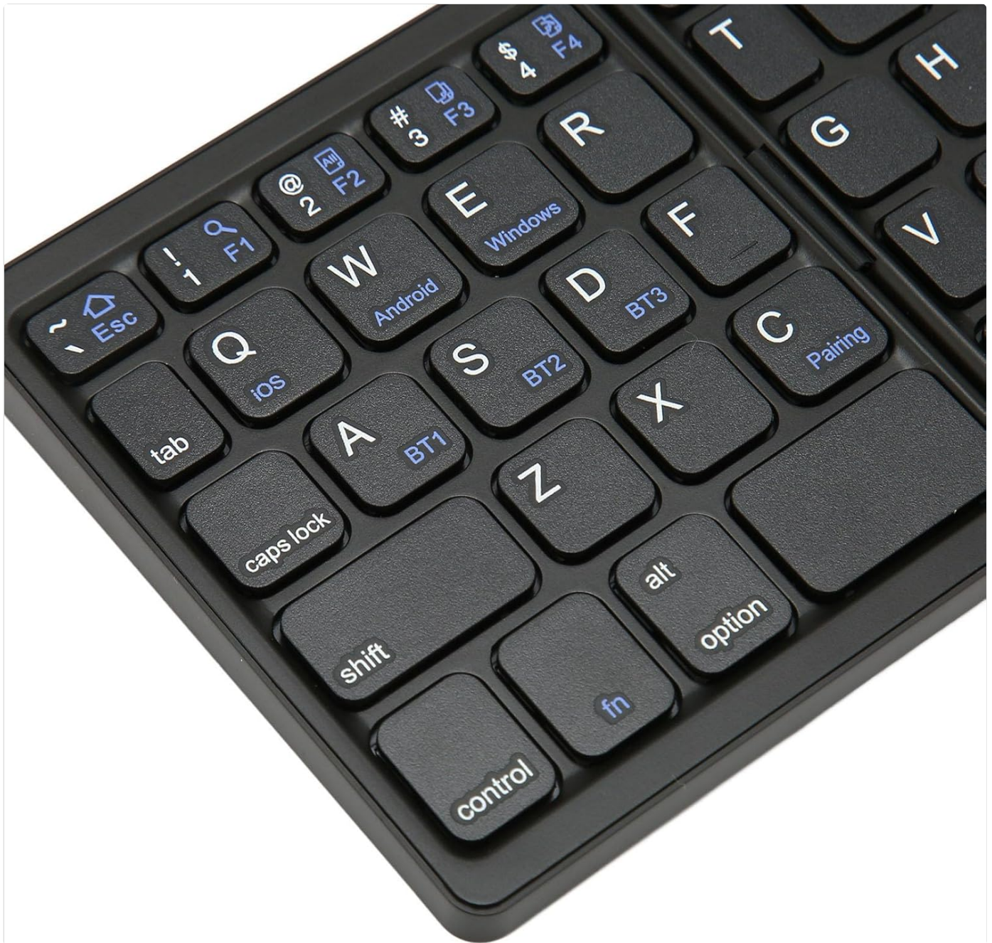
Figure 5.2: Detail of the keyboard's left section, highlighting the operating system specific keys (iOS, Android, Windows) and the Bluetooth channel keys (BT1, BT2, BT3) used for pairing and switching devices.
