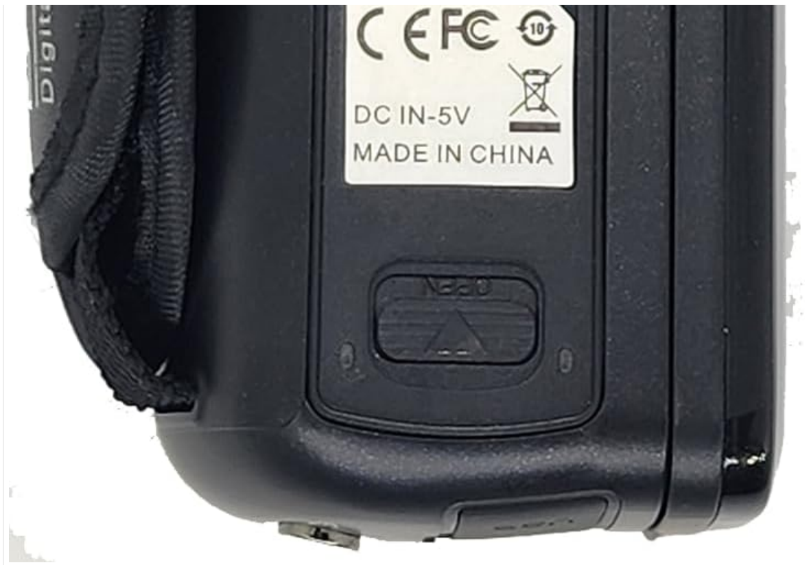
Figure 3: Bottom view of the camcorder, highlighting the battery and SD card access.
