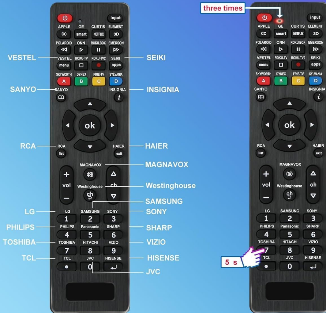
Figure 3.1: Brand Setting Method. This diagram visually explains how to program the remote by holding down the specific brand button for 5 seconds until the LED flashes three times.
