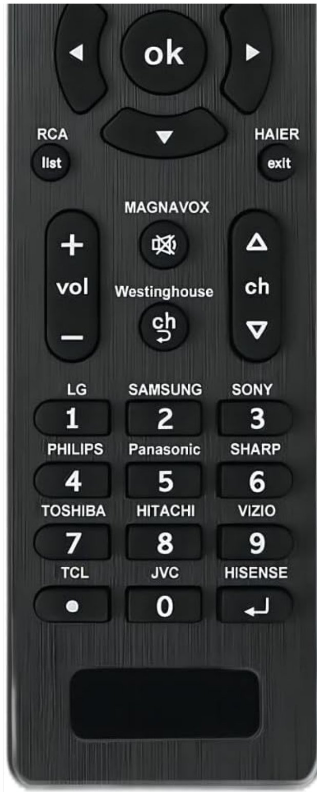
Figure 2.1: Front view of the RC-G008 Universal Remote Control. This image displays the entire remote, highlighting the power button, input button, navigation pad, volume and channel controls, and dedicated brand buttons for various TV manufacturers.
