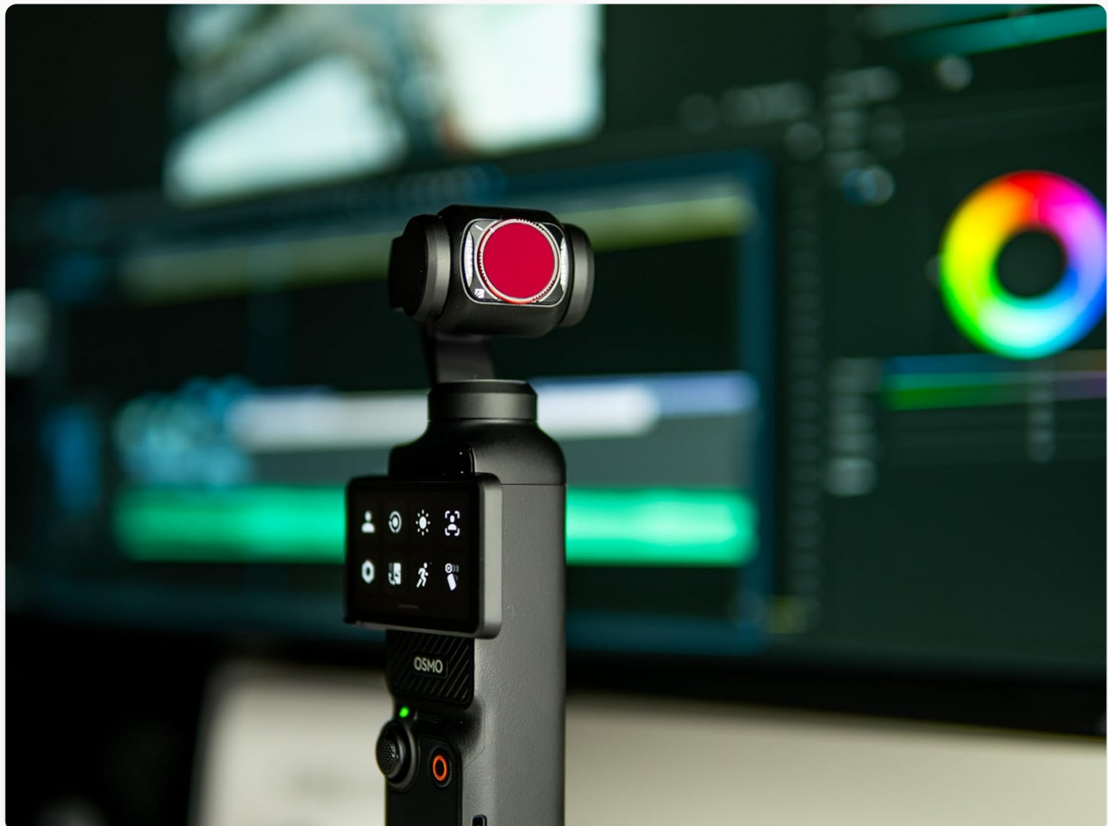
Figure 2: A Freewell ND/PL filter magnetically attached to the Osmo Pocket 3 lens, ready for use.
