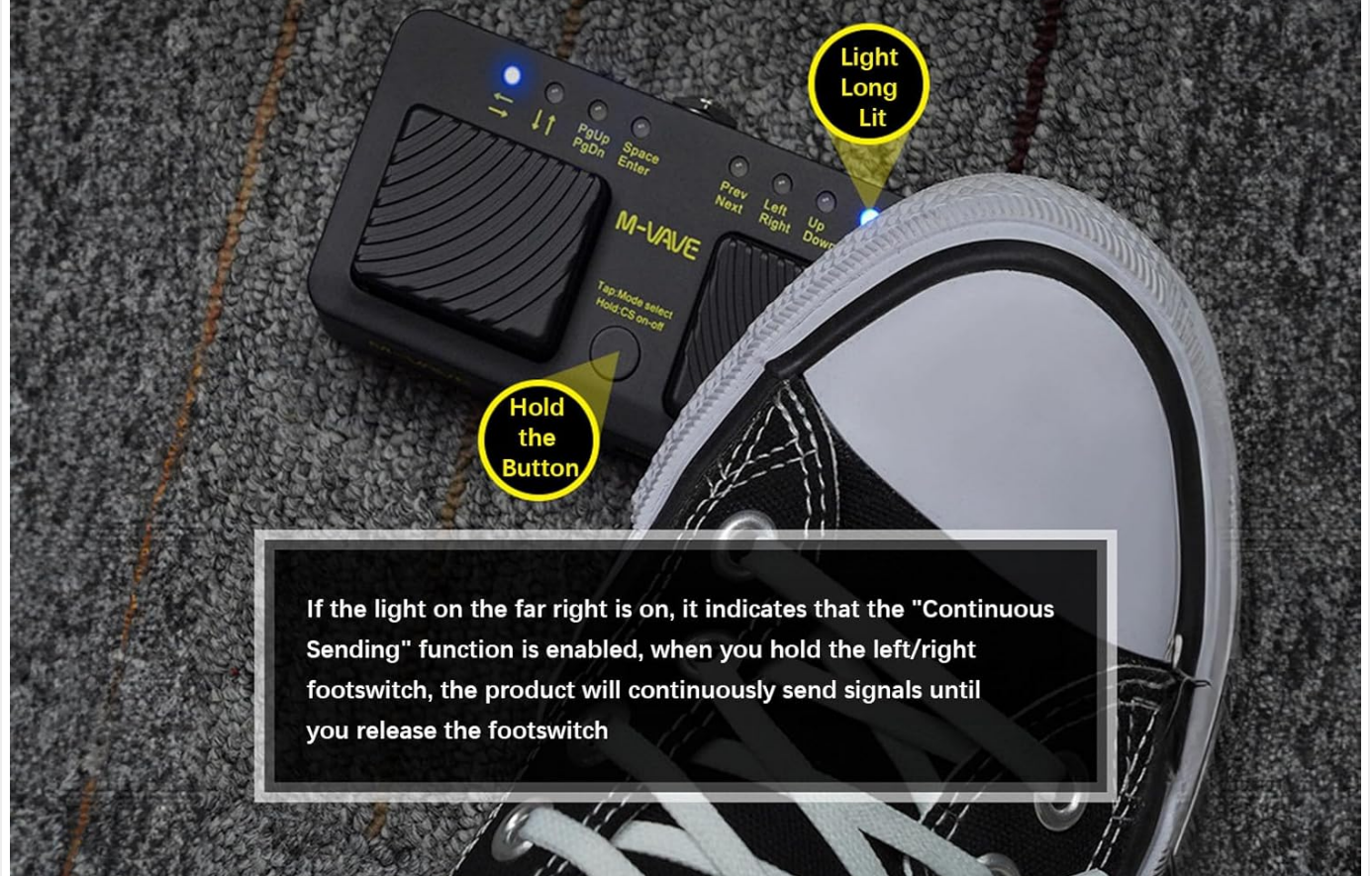
Figure 5.1: Continuous Sending Feature. This image highlights the indicator light for the 'Continuous Sending' function and explains how holding down a footswitch enables continuous signal transmission.
