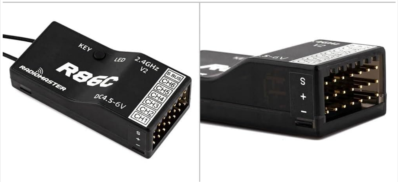
Top-down view of the RadioMaster R86C V2 receiver, highlighting the 'KEY' button, 'LED' indicator, '2.4GHz V2' label, 'DC4.5-6V' power input, and clearly labeled channel outputs (S.BUS, CH6-CH1).
