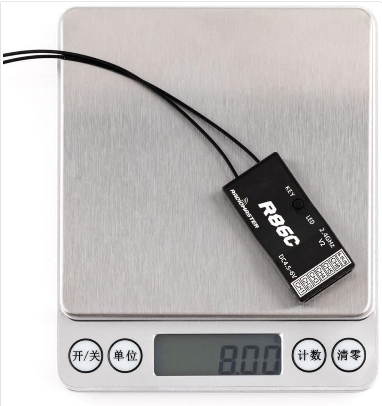
The RadioMaster R86C V2 receiver placed on a digital scale, displaying a weight of 8.00 grams.
