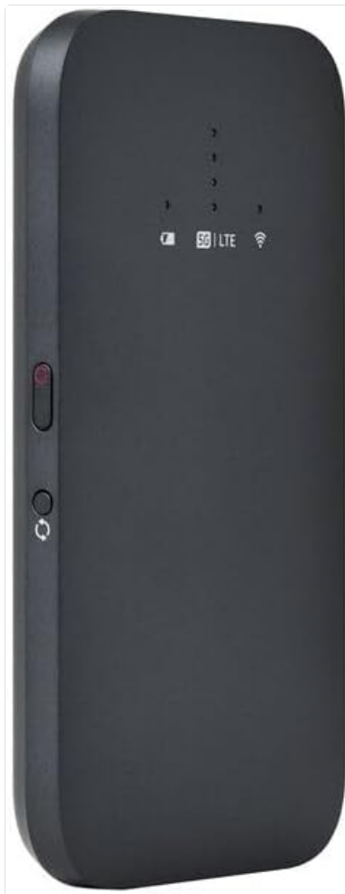
Figure 5: Angled front view of the mobile hotspot, clearly showing the LED indicators for battery, 5G/LTE, and Wi-Fi.
