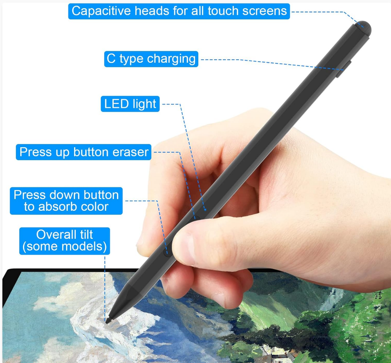
Image 3.1: Diagram illustrating the stylus features, including capacitive heads, USB-C charging port, LED light, up button (eraser), and down button (color absorption/right-click).
