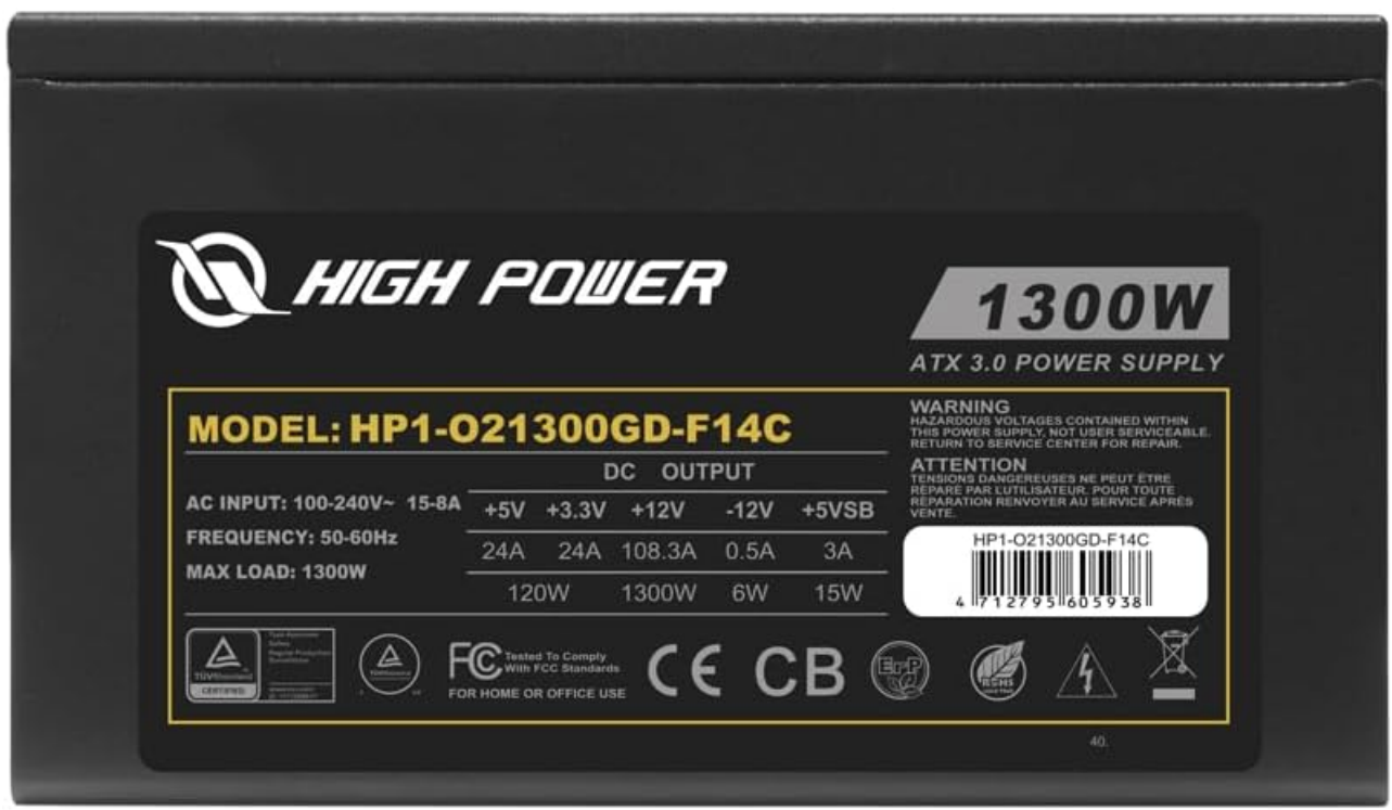
Image: The product label displaying detailed electrical output specifications for the High Power 1300W ATX 3.0 Power Supply.
