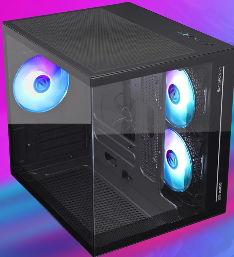
Figure 3: Overview of pre-installed fans and locations for additional AIO cooler mounting.
