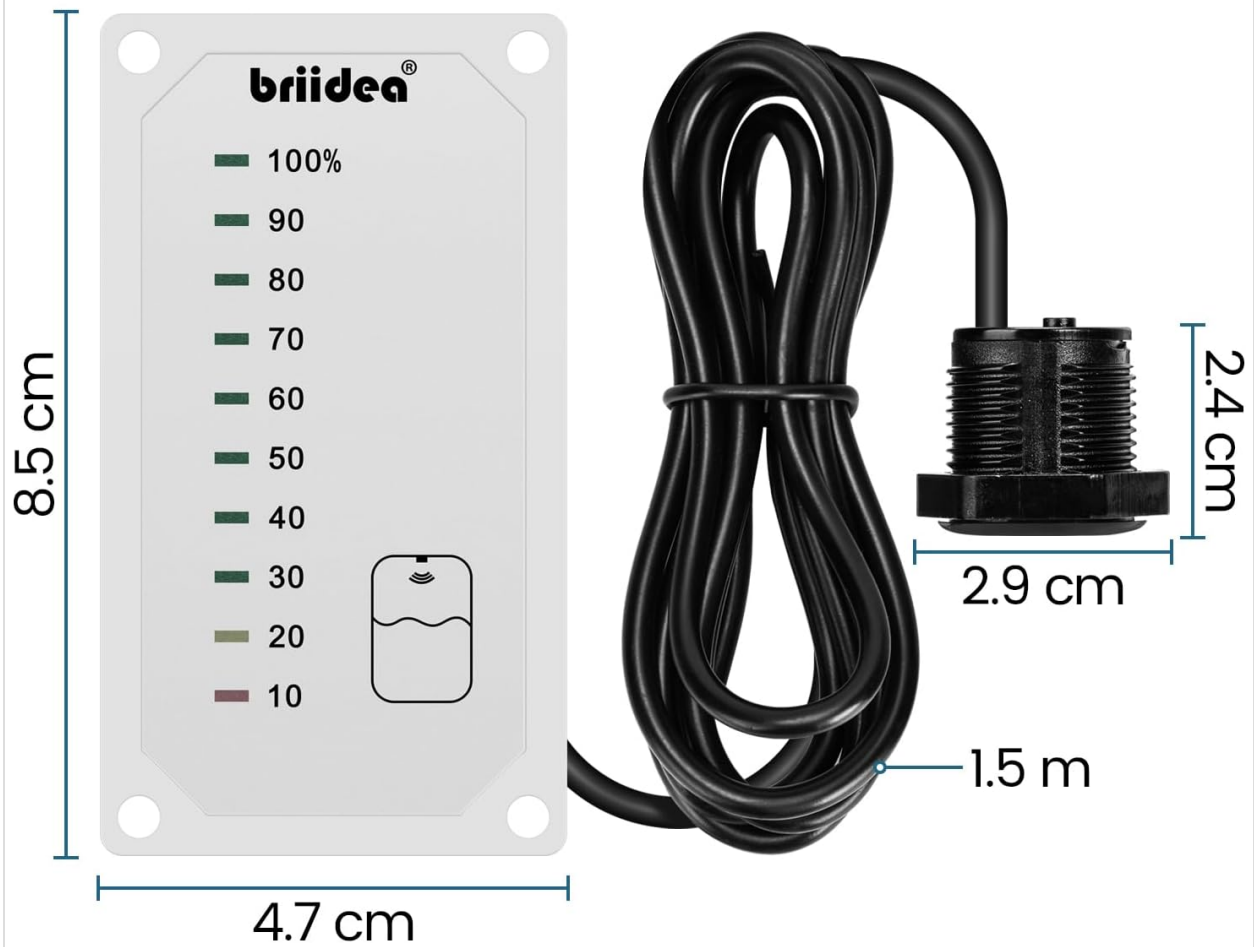
Figure 6: Product Dimensions. This image provides the physical dimensions of the indicator panel (8.5 cm height, 4.7 cm width) and the sensor (2.9 cm diameter, 2.4 cm height) with a 1.5 m cable.
