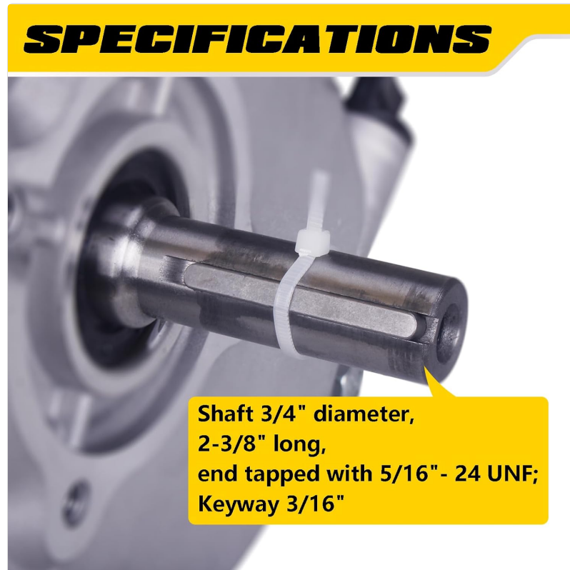
Figure 3: Detailed view of the engine shaft specifications.
