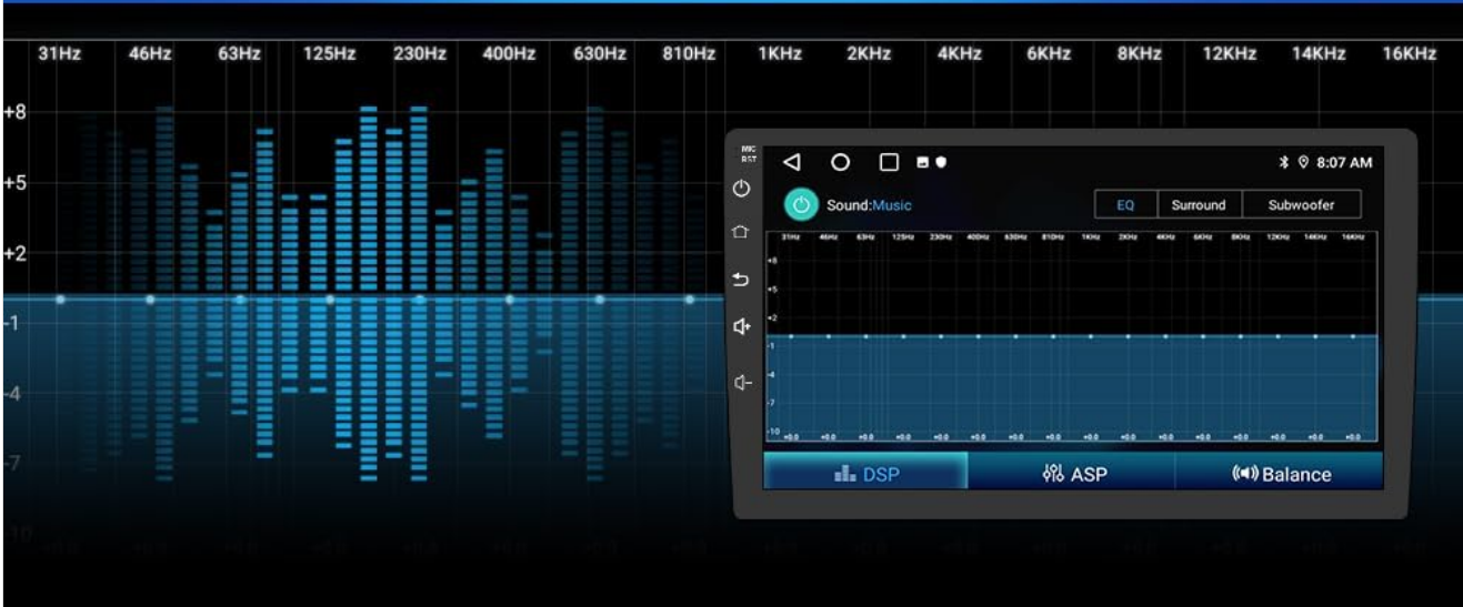
Image: The Junsun head unit displaying the Digital Signal Processing (DSP) interface with a graphic equalizer for audio adjustments.
