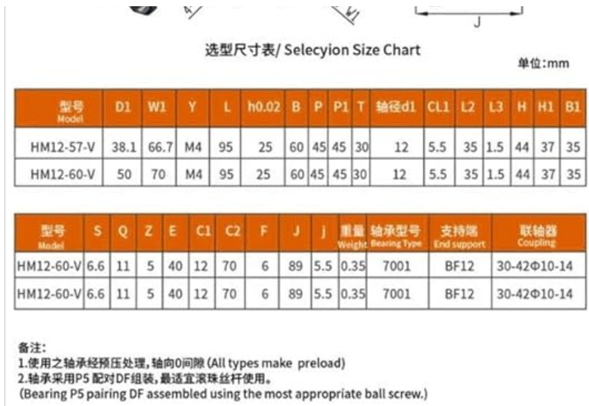
Figure 5: Technical diagram for HM12-57 and HM12-60 series mounts, including dimensions and assembly details.
