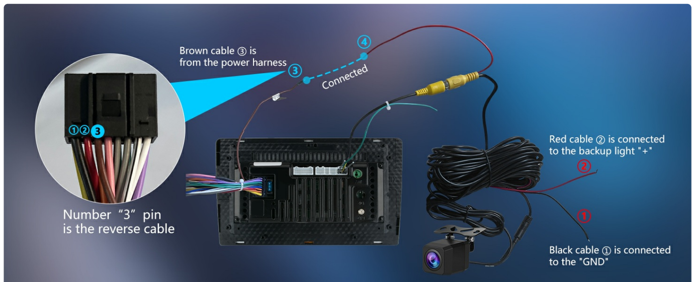
Image: A diagram detailing the proper connection of a rear camera to the head unit, including the reverse trigger wire.
