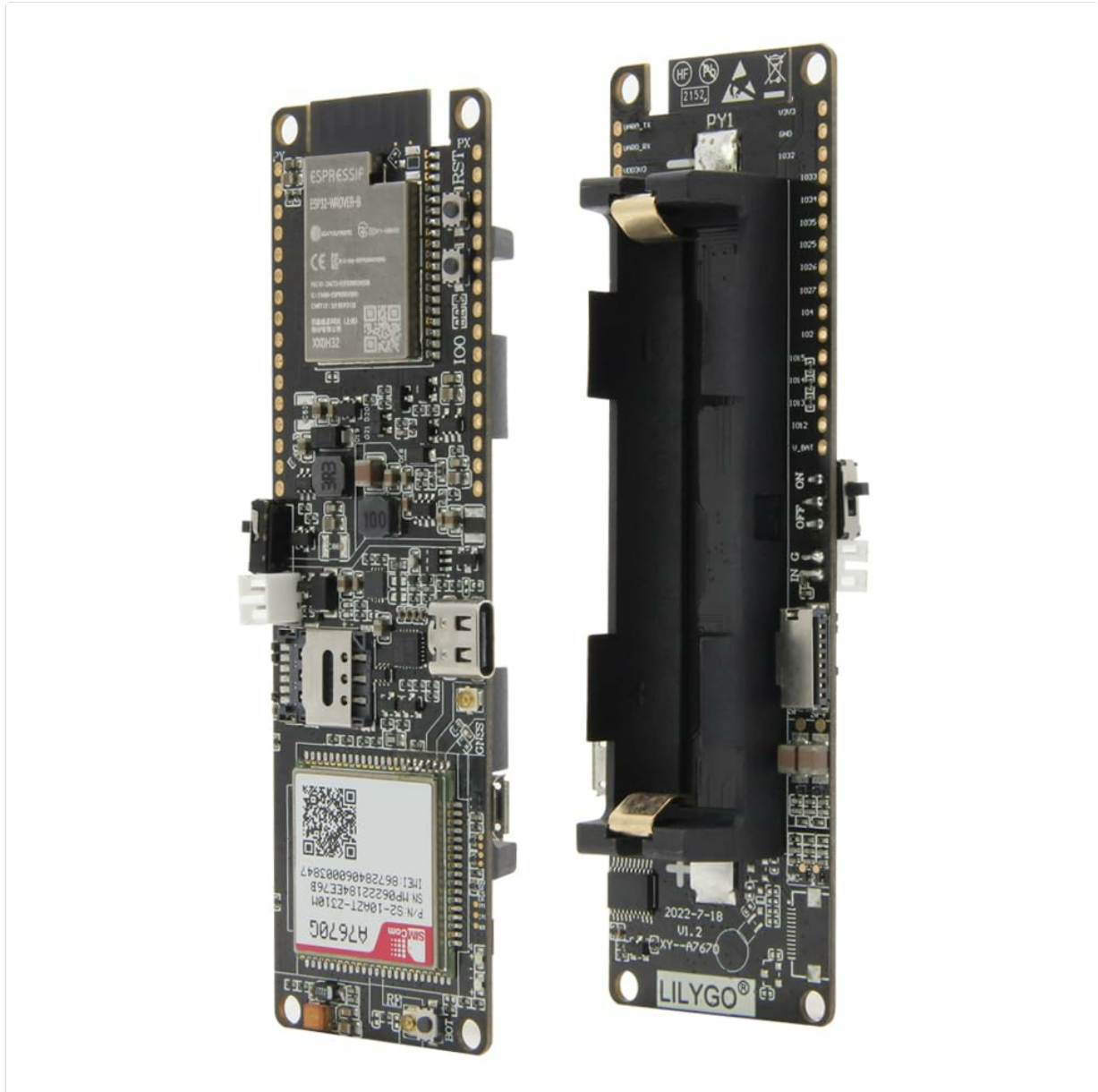
Image: Top view of the LILYGO T-A7670G R2 development board, showing the ESP32-S3 module, SIM7670G module, USB-C port, and SIM/TF card slots.
