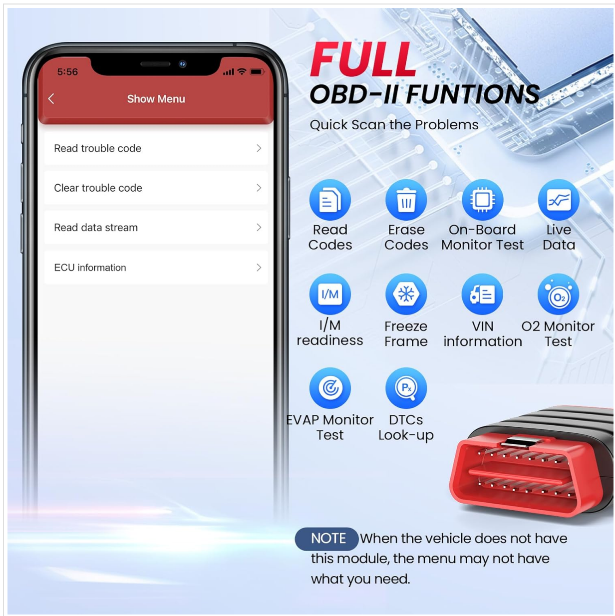
Image: A screenshot of the THINKDIAG app interface detailing the full suite of OBD-II functions available, such as Read Codes, Erase Codes, Live Data, and O2 Sensor Test.
