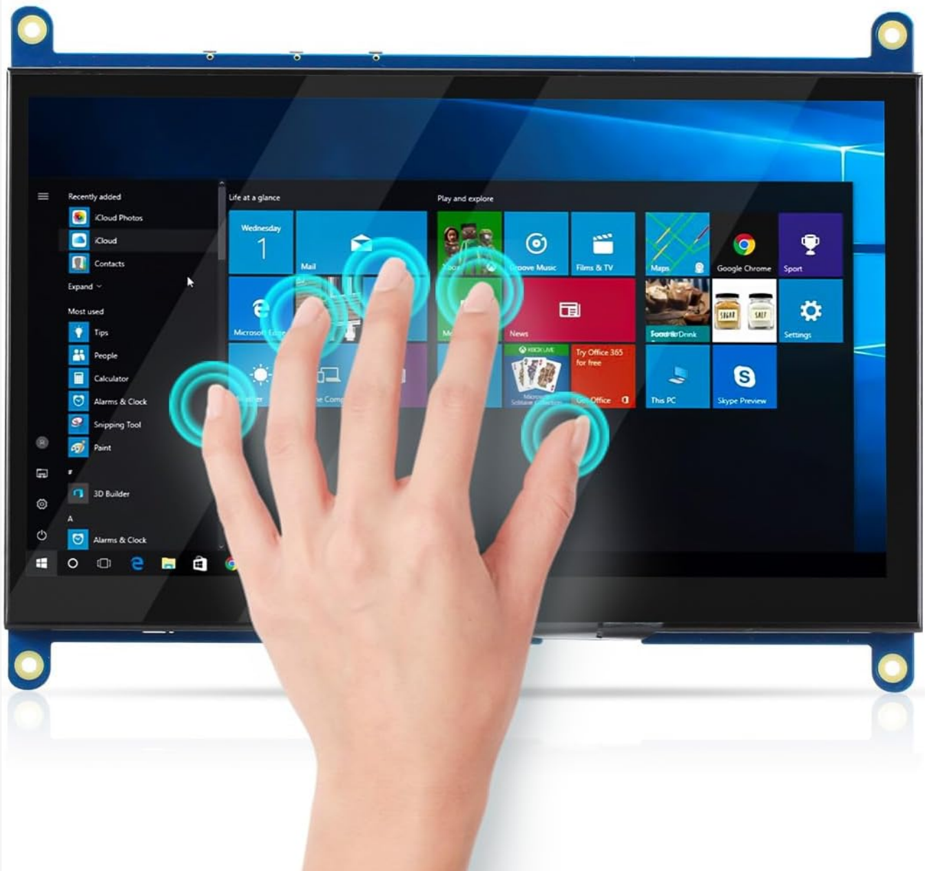
Figure 4: 5-Point Capacitive Touch. This image demonstrates various touch gestures supported by the monitor, including single touch, zoom in, zoom out, drag, and rotation, highlighting its responsive and multi-touch capabilities.
