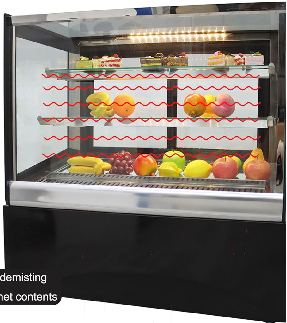
Figure 3.4: Demonstration of the demist function, which uses an electric heating wire to prevent fogging on the front glass, ensuring clear product visibility.
