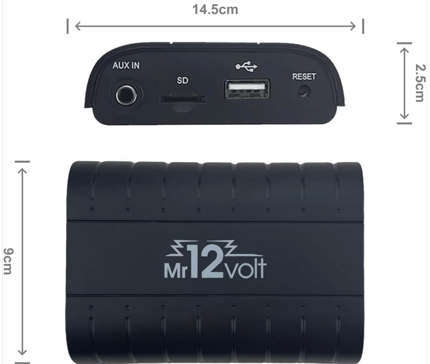
Image: Diagram showing the dimensions of the MR 12 VOLT module: approximately 14.5cm in length, 9cm in width, and 2.5cm in height, useful for planning installation space.
