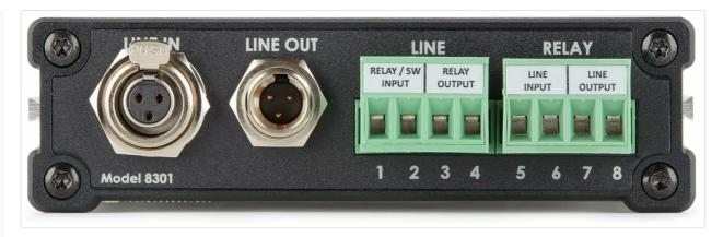
This image shows the rear panel of the ALGO 8301, highlighting its connectivity options. From left to right, it features a 'LINE IN' XLR connector, a 'LINE OUT' XLR connector, and two terminal blocks labeled 'RELAY / SW INPUT', 'RELAY OUTPUT', 'LINE INPUT', and 'LINE OUTPUT' for various audio and control connections. The model number '8301' is also visible.
