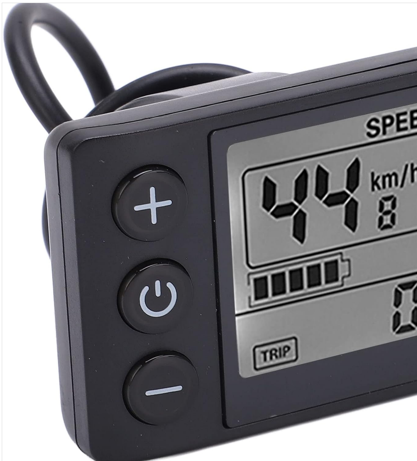
Image: Close-up view of the S866 LCD Display's control buttons: Plus (+), Power (circle with vertical line), and Minus (-).
