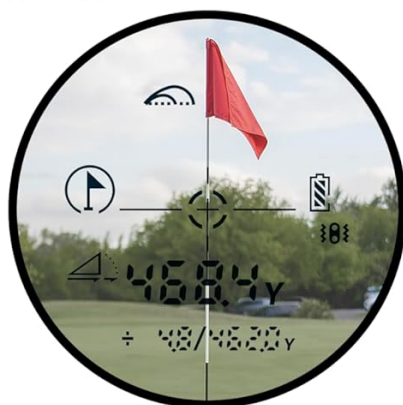
Image 4.2: Illustration of the slope compensation feature on the CIGMAN CT-800Y Golf Rangefinder.
