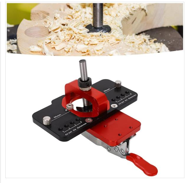
This image highlights the markings on the jig for setting the hinge offset, allowing for precise drilling at 3mm, 4mm, 5mm, or 6mm from the edge of the workpiece.
