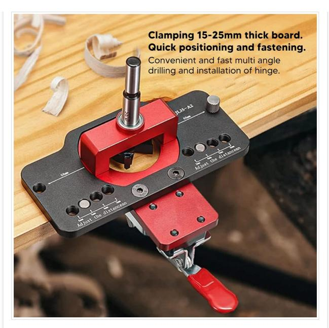
This image demonstrates the jig properly positioned and clamped onto a wooden panel, indicating readiness for the drilling operation.
