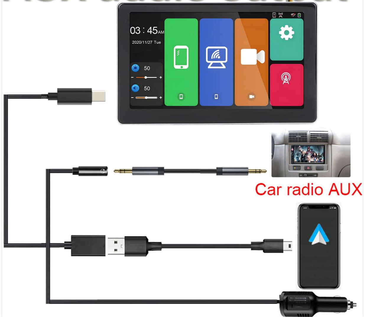
Figure 4.4: Connection diagram for AUX audio output, detailing how to link the dash cam to a car's audio system using an AUX cable for direct sound transmission.
