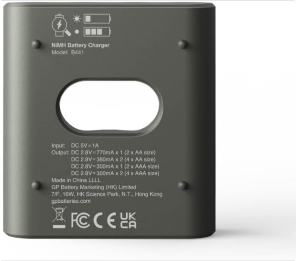
Figure 9.1: Bottom view of GP B441 Battery Charger displaying technical specifications and regulatory marks.
