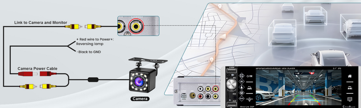
Figure 3.3: Visual representation of the reversing camera connection and its display on the car stereo.
