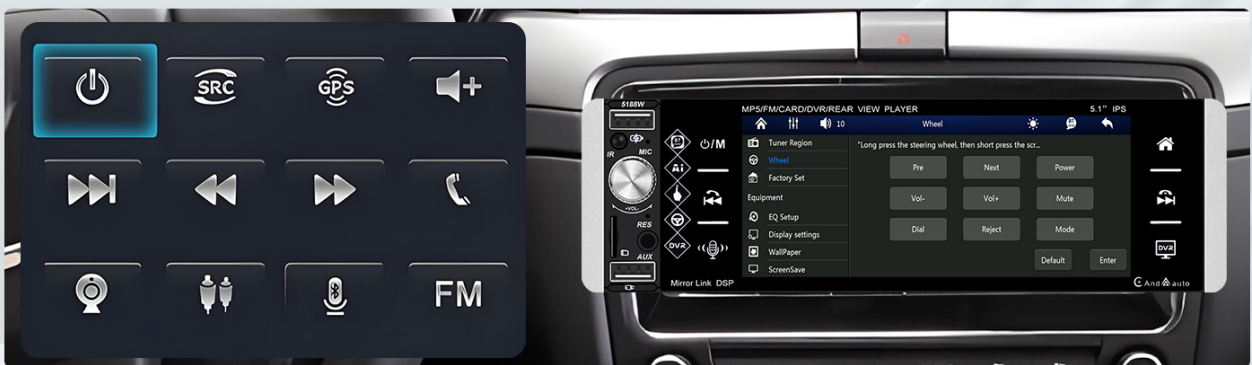
Figure 4.9: Steering Wheel Control setup interface.
