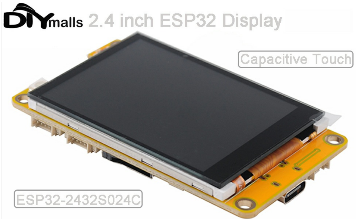
Figure 1: Overview of the ESP32-2432S024C development board, highlighting key components such as the ESP-32 module, TF card slot, Type-C USB port, and various connectors for power, battery, speaker, and external I/O.
