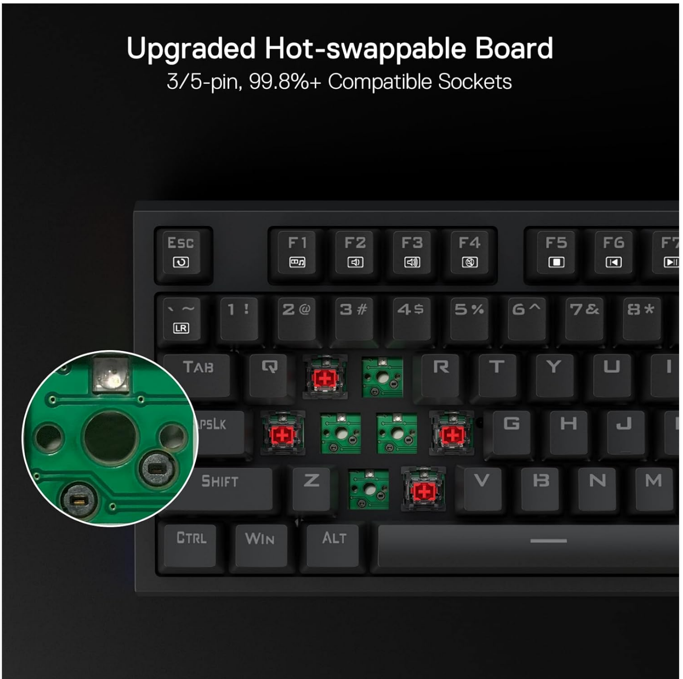
Image: A close-up view of the hot-swappable sockets on the Redragon K670 keyboard with switches removed.
