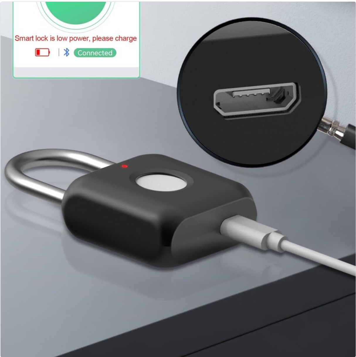
Image: The padlock being charged via its USB port. A red light indicates charging, and the app displays "Smart lock is low power, please charge" and "Connected" status.
