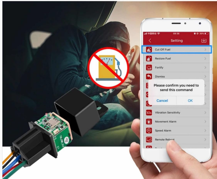
Figure 5.2: The mobile application displaying the remote fuel cut-off function, a security feature to disable the vehicle's engine remotely.
