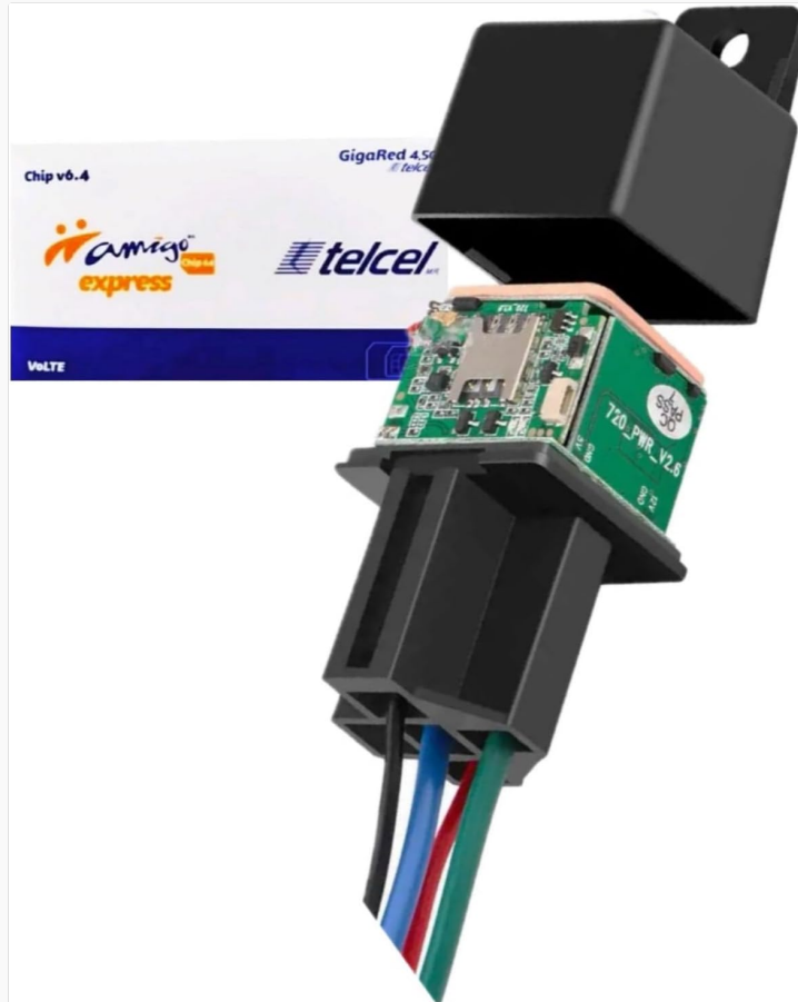
Figure 2.1: The Micodus MV720 GPS Tracker, designed to look like a vehicle relay, shown with a SIM card package.
