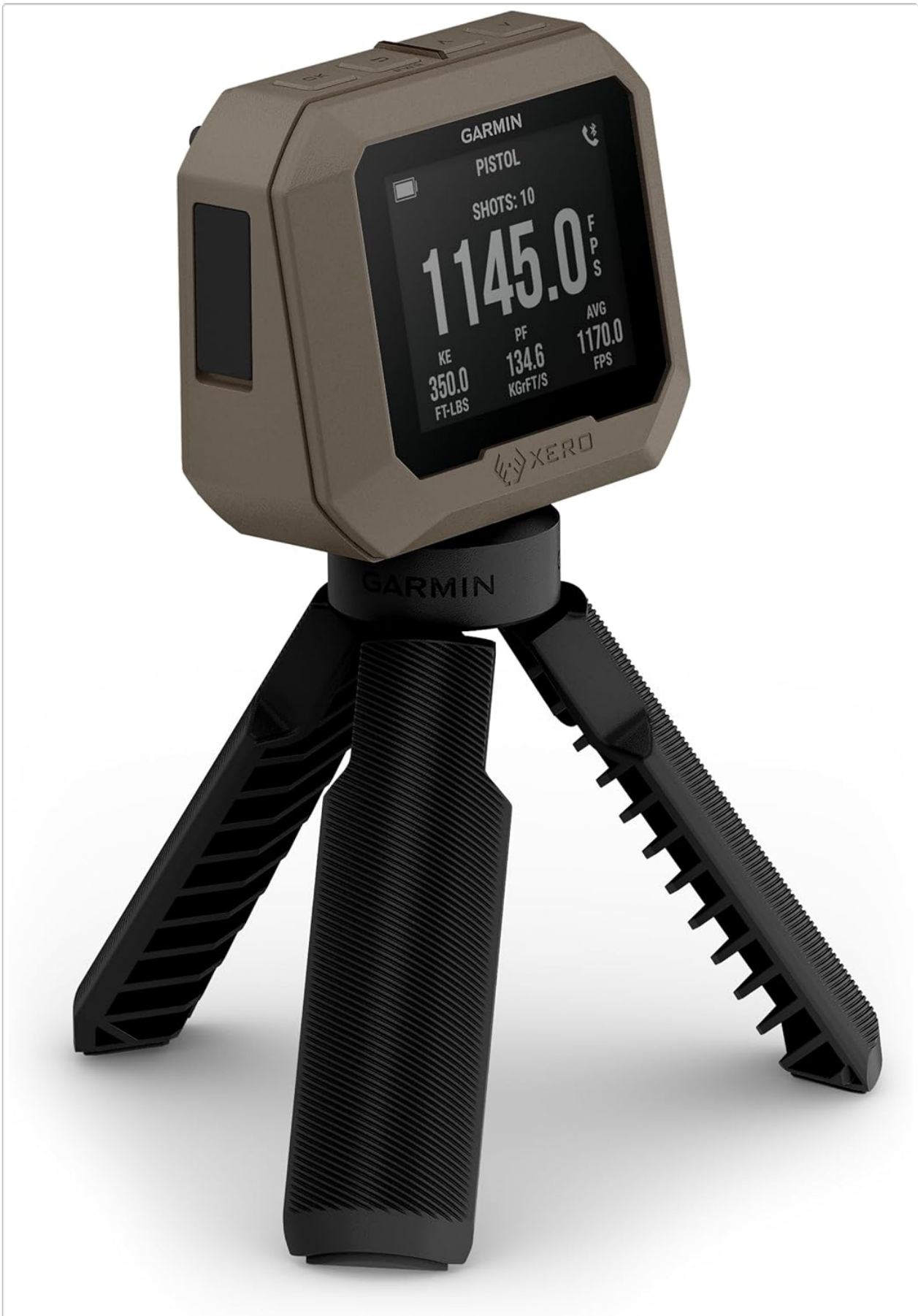
Image 5.2: The Xero C1 Pro display showing a velocity measurement in Pistol mode, including kinetic energy and power factor.
