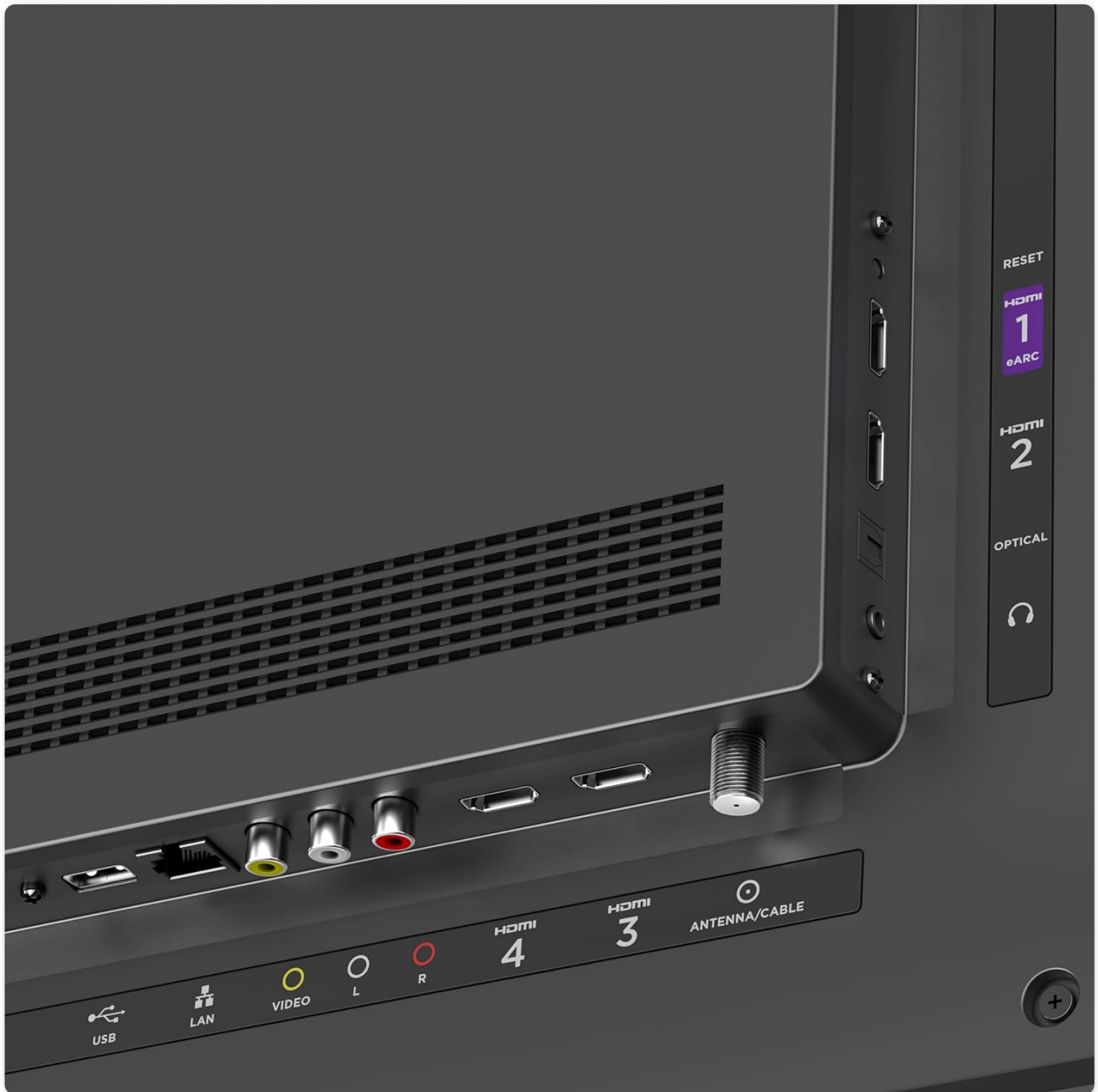
Image: A detailed view of the rear panel of the Roku TV, highlighting the various input and output ports including HDMI, USB, Optical, and Ethernet.
