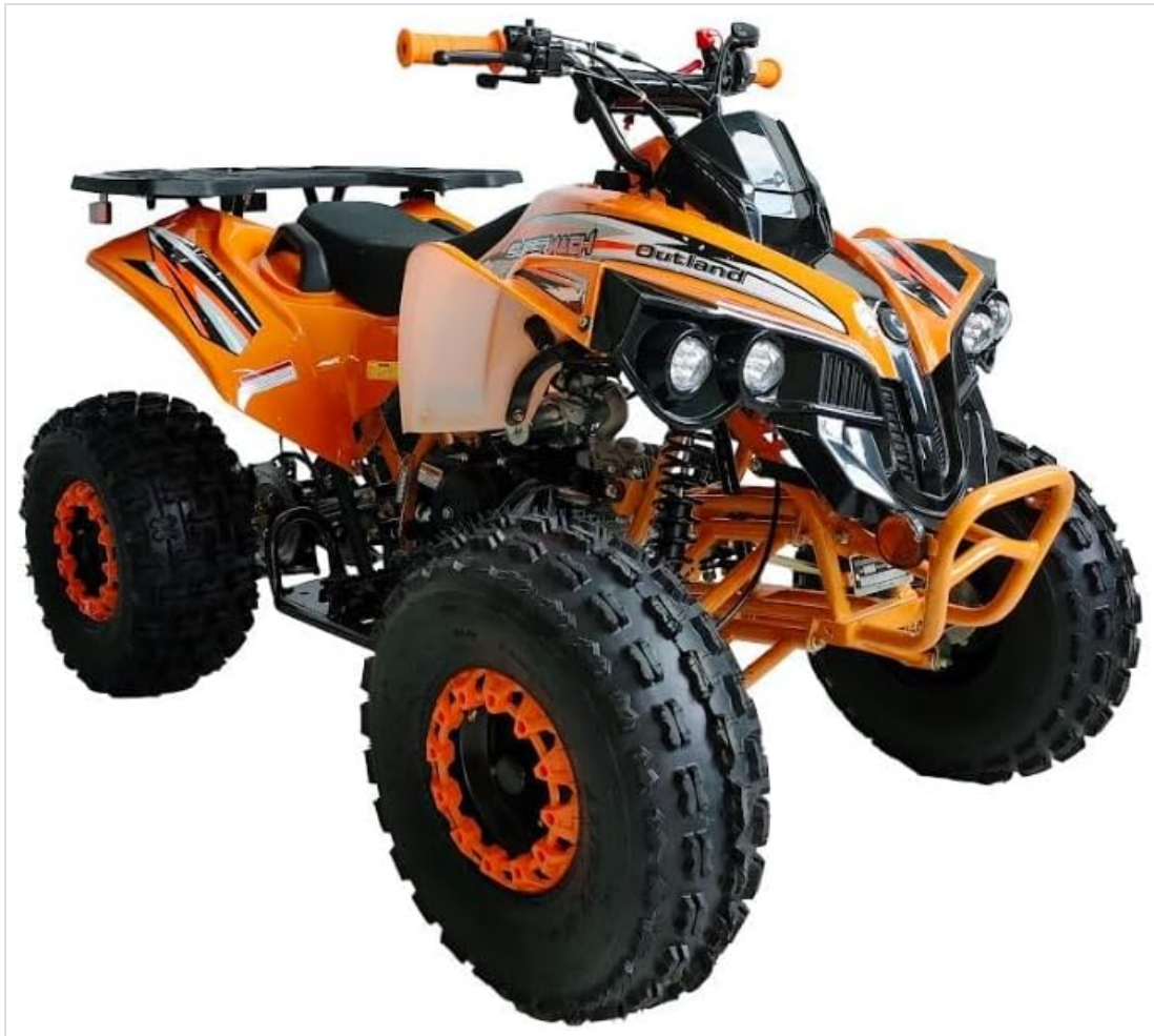
Front view of the HHH 125cc ATV, highlighting the installed front bumper.
