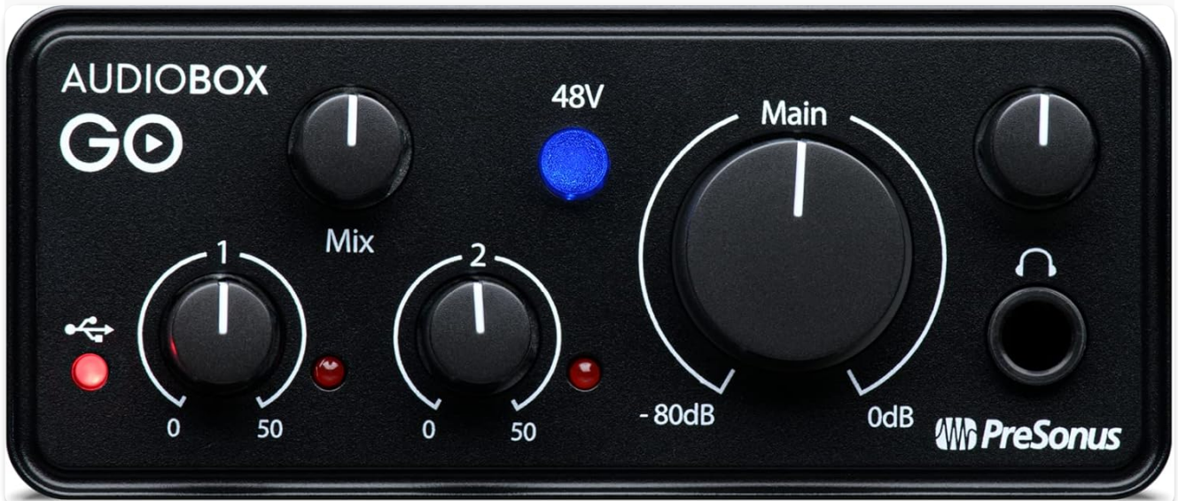
Image 2: Front panel of the PreSonus AudioBox GO, showing input jacks, gain controls, and monitoring options.
