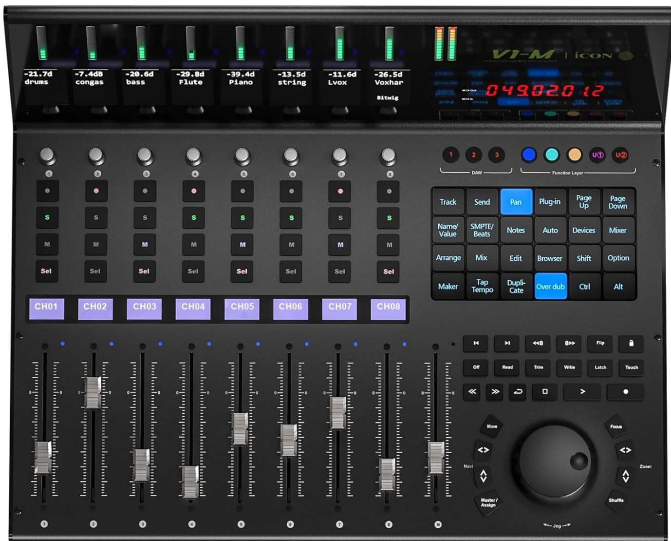
Figure 4: Top-down view of the V1-M, illustrating the layout of faders, encoders, and channel controls.
