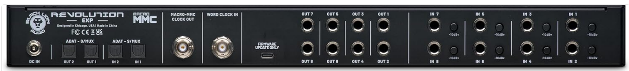
Figure 3.2: Rear panel of the Revolution EXP, displaying DC IN, ADAT I/O, Word Clock I/O, and analog TRS I/O connections.
