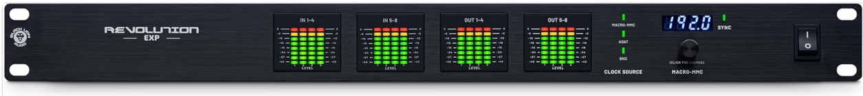
Figure 3.1: Front panel of the Revolution EXP, showing input/output meters, clock source selection, and power switch.
