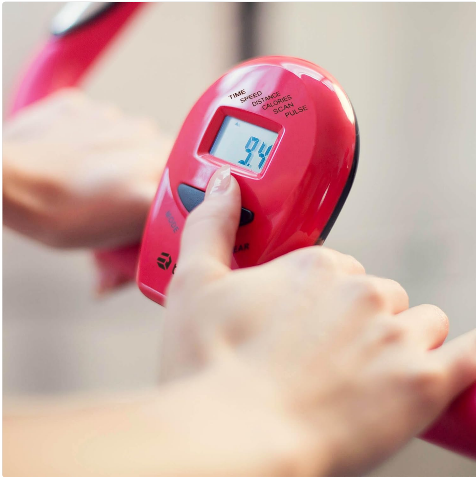
Figure 4.2: Close-up of the training computer display. This image shows the LCD screen which displays various metrics such as time, speed, distance, calories, and pulse, along with the 'Mode' and 'Reset' buttons.
