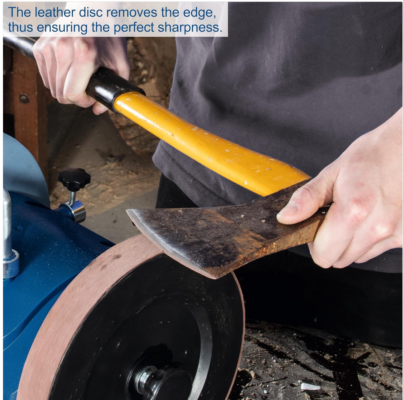
Image 5.2: The leather disc removes the burr, ensuring a perfectly sharp edge.
