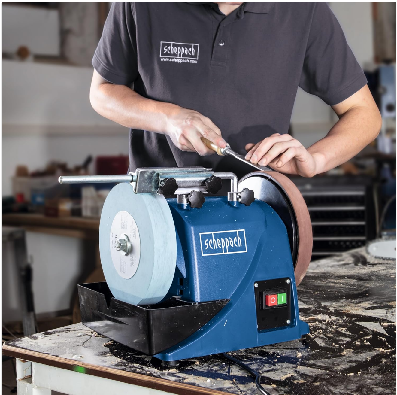
Image 5.1: Sharpening a chisel using the universal grinding jig for precise angle control.
