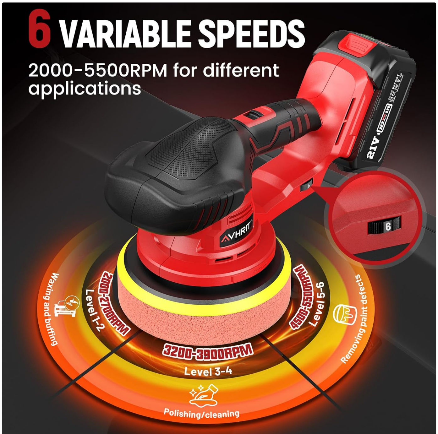
Figure 4: Diagram illustrating the 6 variable speed settings and their recommended applications: Level 1-2 (2000-2700 RPM) for waxing and buffing; Level 3-4 (3200-3900 RPM) for polishing/cleaning; Level 5-6 (4500-5500 RPM) for removing paint defects.
