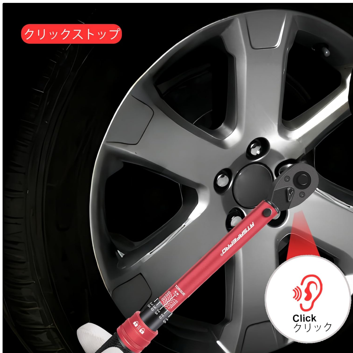
Image 5.2: Illustration of the audible 'click' feedback when the target torque is achieved.
